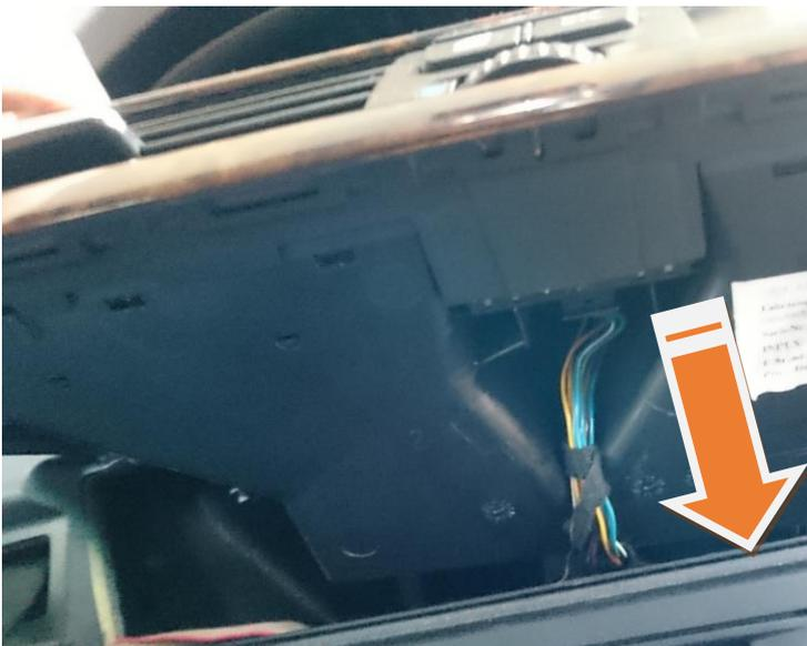
For some models, the switch unit can now be pushed out from back to front (i.e. E91). For others (i.e. E92), the fresh air grill must first be disconnected from the interior trim (next item).
