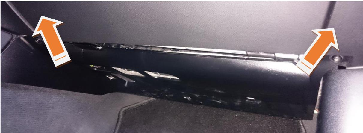
Now the cover can be carefully drained. Attention, there is still a plug connection of the footwell lamp to separate.
