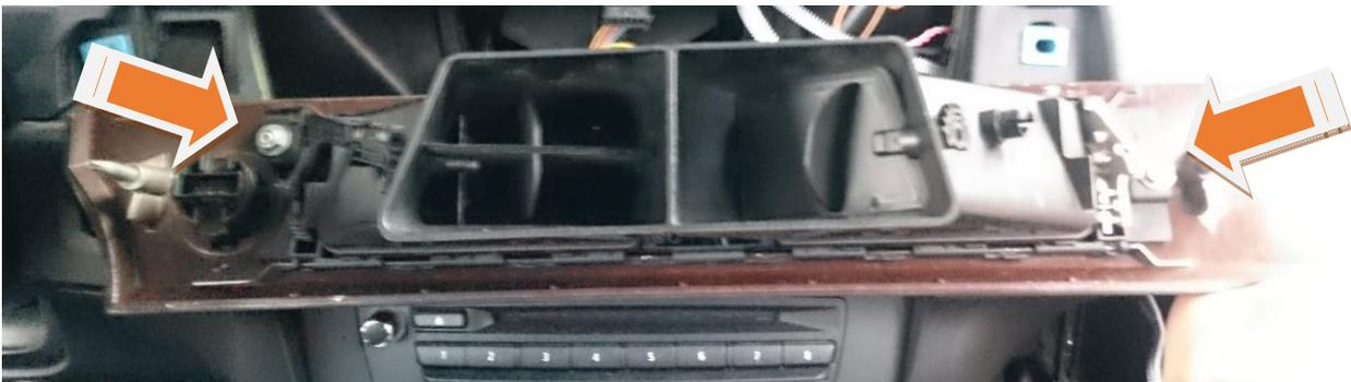
The clips must be unlocked carefully with a flat-head screwdriver.
