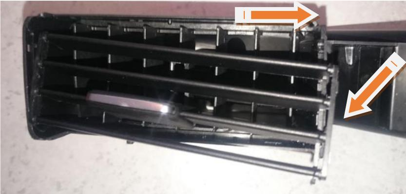
To remove the other part, the housing must be gently pushed apart.
