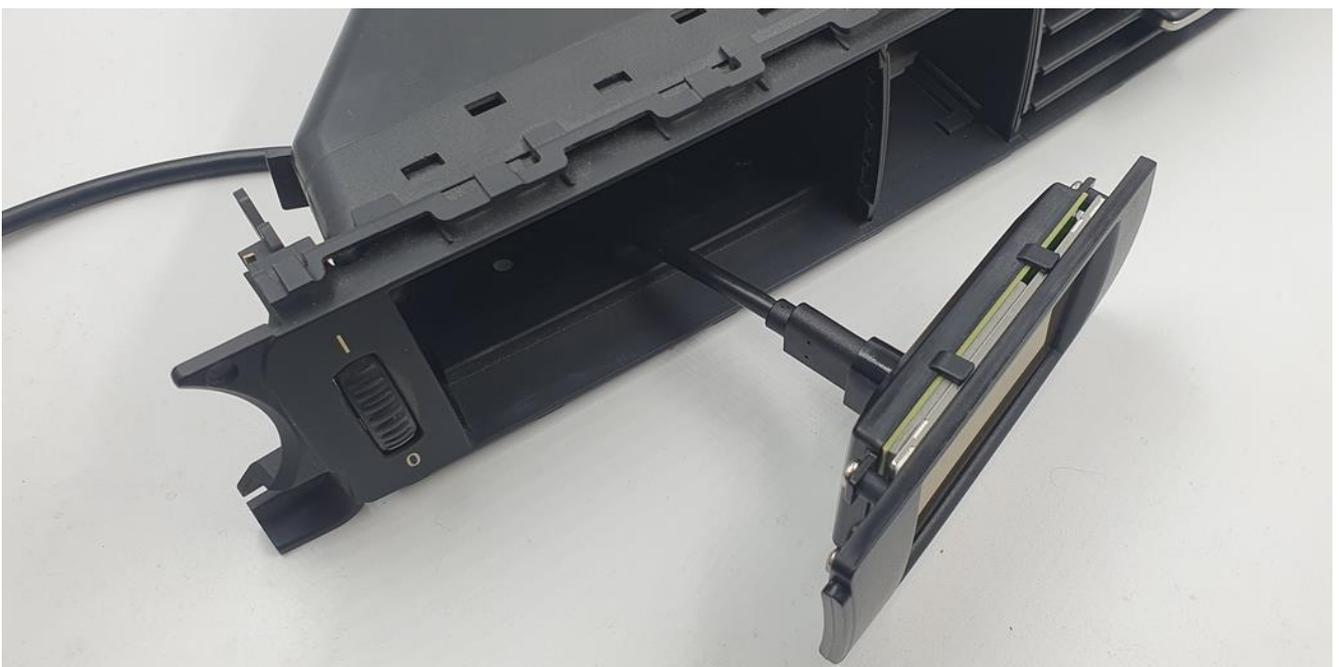
Carefully slide the display sideways behind the panel and press the display. The other side will later be held by the hazard warning switch.
