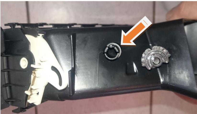
The next step is to separate the front panel of the fresh air grill from the case.
